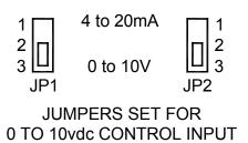
The IPT has been adjusted at the factory for a 4 to 20 madc or 0 to 10 vdc control input signal to produce a 0 to 80 psig output pressure. No further adjustments are required. However, if adjustment of the output pressure is desired, see note below.
